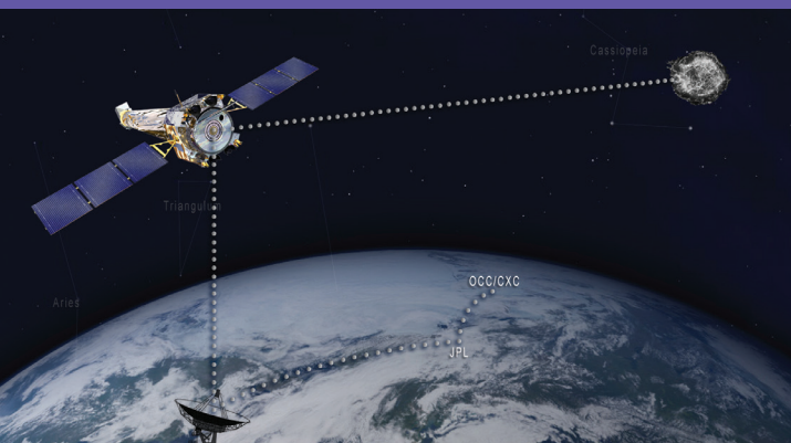
The data path from the cosmic source, to the satellite, to Earth. The data transmitted in binary code before being translated into a visual representation of the object. Credit: NASA/CXC/SAO
