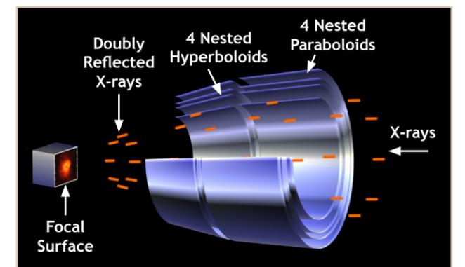
Illustration of the design and functioning of the High Resolution Mirror Assembly (HRMA) on Chandra. X-rays that strike a mirror head-on are absorbed, while X-rays that hit a mirror at grazing angles are reflected like a pebble skipping across a pond. Thus, X-ray telescope mirrors are shaped like barrels rather than dishes, where the X-rays reflect off the inner, polished surfaces and are focused onto a detector to produce an image.
